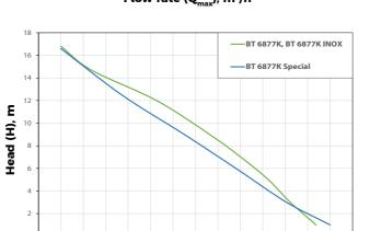
Flow rate (Q<sub>max</sub>), m<sup>3</sup>/h
