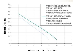
Flow rate (Q<sub>max</sub>), m<sup>3</sup>/h
